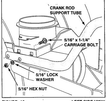
Attach the chute tilt control assembly to the top side of the crank support tube using two 5/16" x 1-3/4" carriage bolts, bowed washers, 5/16" lock washers and 5/16" hex nuts. See figure 19.
